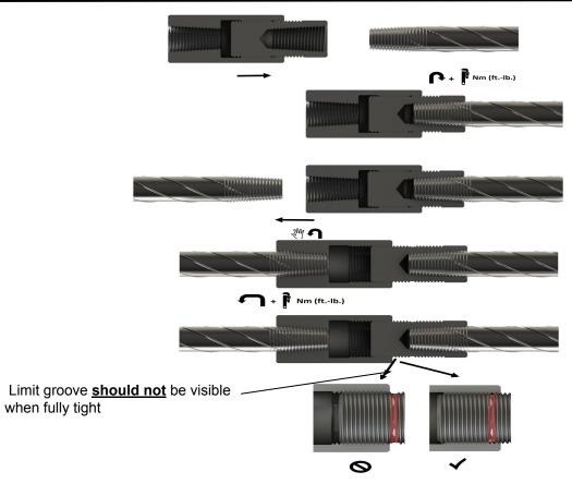
NOTE :Couplers must be assembled with calibrated torque wrench. Torque wrench must be calibrated at least every 24 months (+/- 15%).
